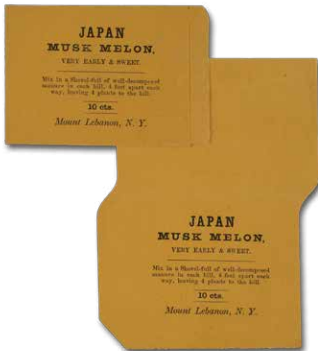
Figure 4: A stack of rectangular printed papers were trimmed with off-set chisels to form flaps that were later folded and pasted.
