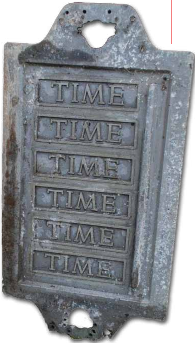
This two-sided 1950s aluminum match plate weighs 17 pounds and measures 27 x 14 x 2 inches.
